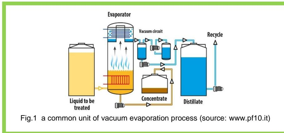
Fig.1 a common unit of vacuum evaporation process (source: www.pf10.it)
