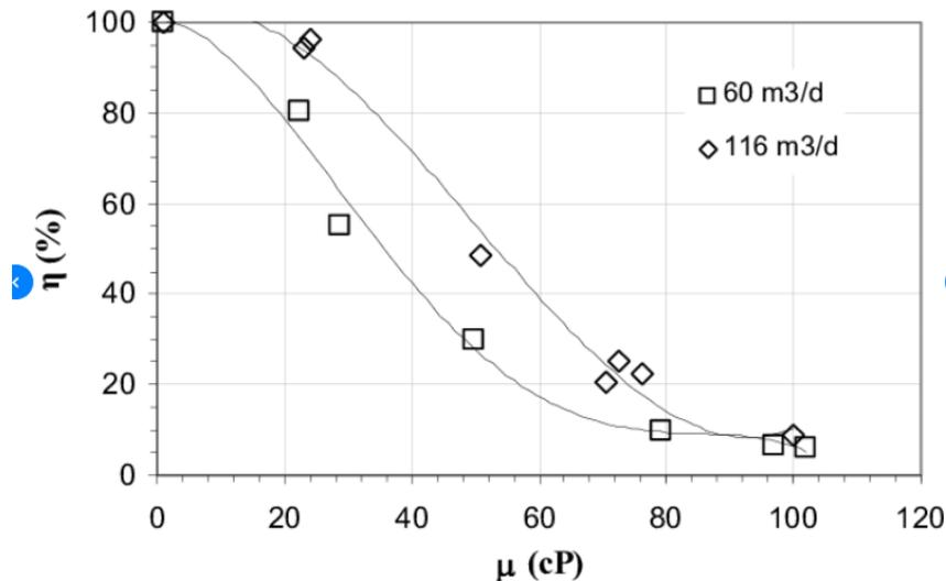
Separation efficiency as a function of the liquid viscosity. The inlet solids concentration and mean diameter were constant and equal to 0.1% and 900  $\mu$ m.
