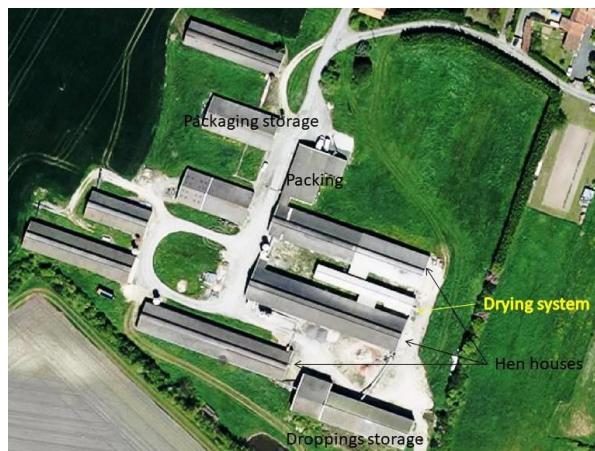
The poultry droppings are collected on treadmills in the hen houses and brought to a drying tunnel. The system uses the heat collected by the ventilation of the air in the hen houses. The transformed poultry droppings are brought with a conveying tunnel in a storage to be mixed and homogenized and to be stocked.
