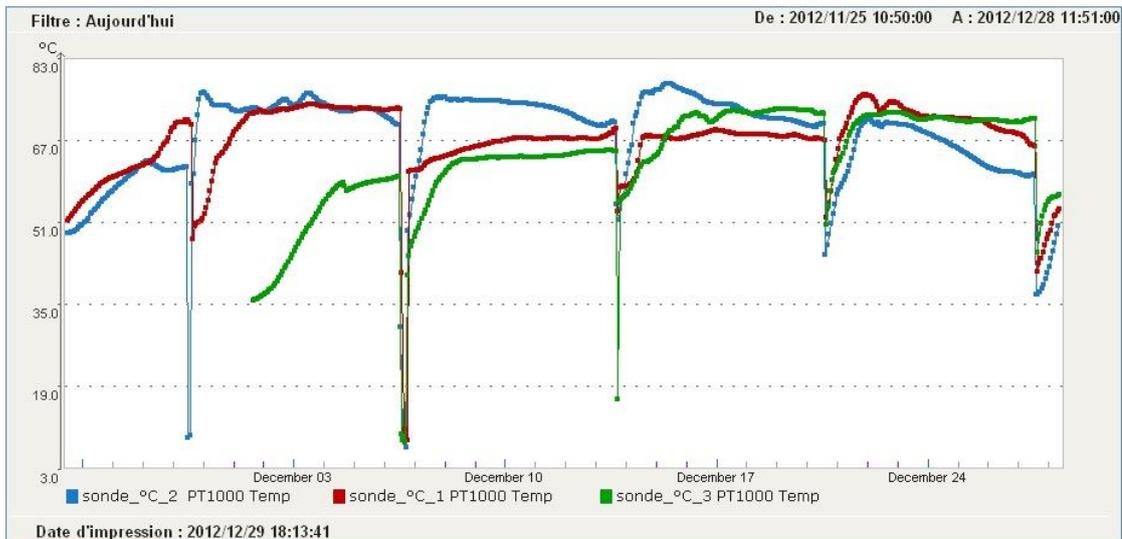
Each coloured curve matches to the temperature monitoring by a different probe on the windrow.
