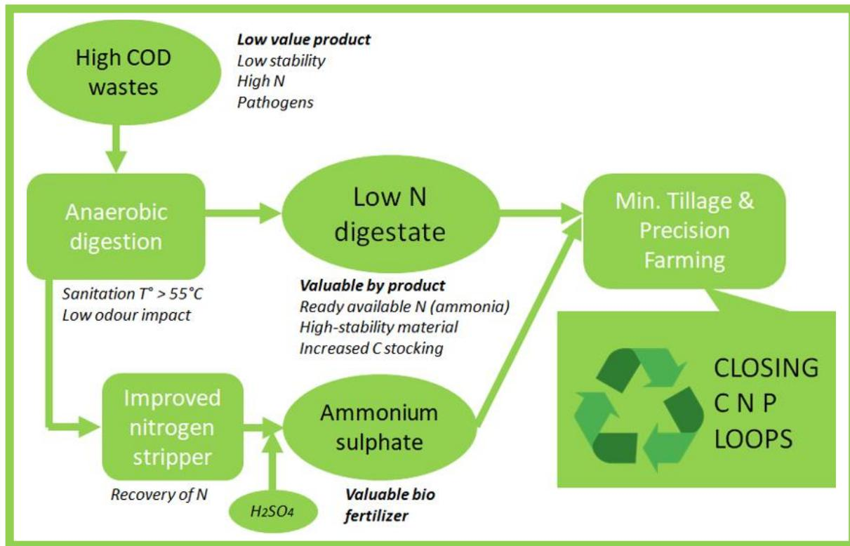
This technique is a complex synergy of technologies to process wastewaters, OFMSW, and agro/food industrial wastes. It includes AD, ammonia stripping system, bio-fertilizer and soils enhancers production, nutrients recycling, precision farming and minimum tillage tools to run effectively rice-culture.
