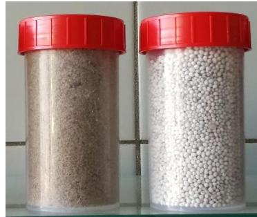
Struvite from sludge and struvite from liquor
