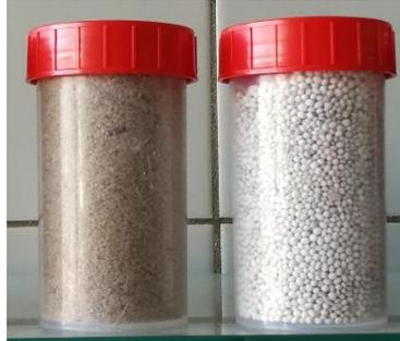
Struvite from sludge and struvite from liquor
