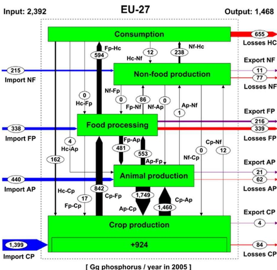
Figure 3.3: Flow diagram of phosphorus in Europe (EU-27) for the year 2005 (van Dijk et al., 2016).
