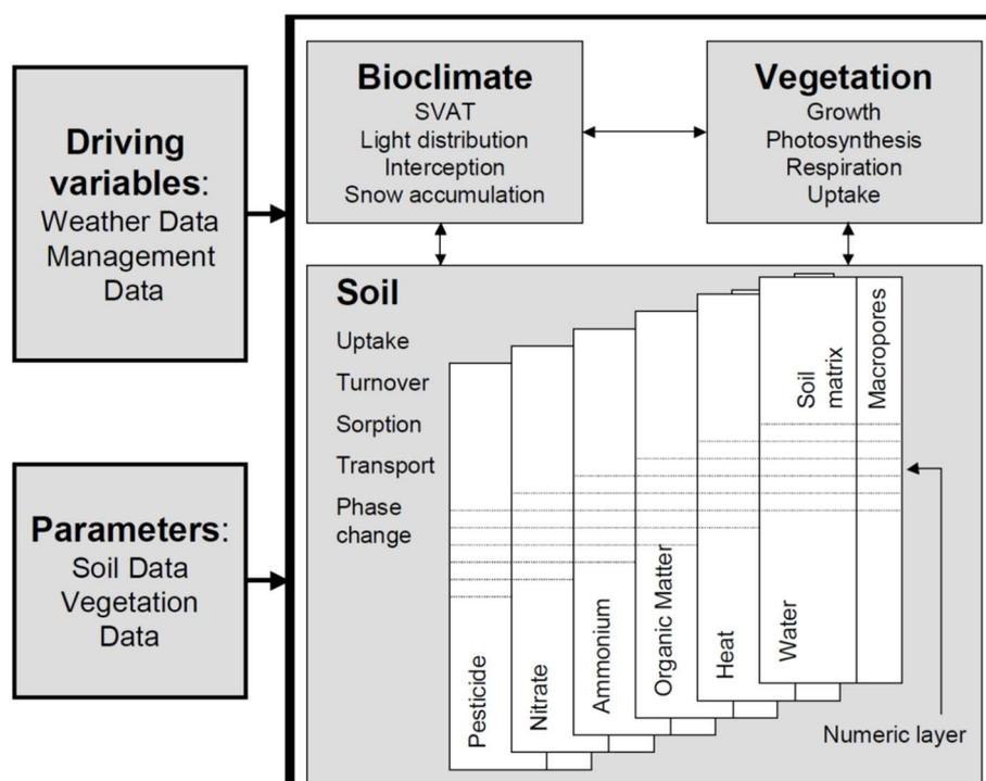
Figure 2.1: Schematic illustration of the Daisy model.
