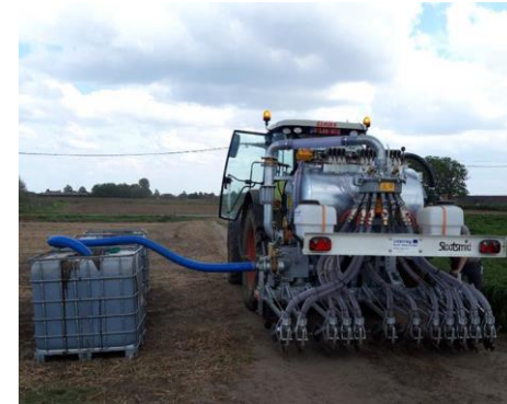
Figure Custom-made fertiliser machine used in field trial (above). Incorporation of fertilisers into top-soil layer (below).
