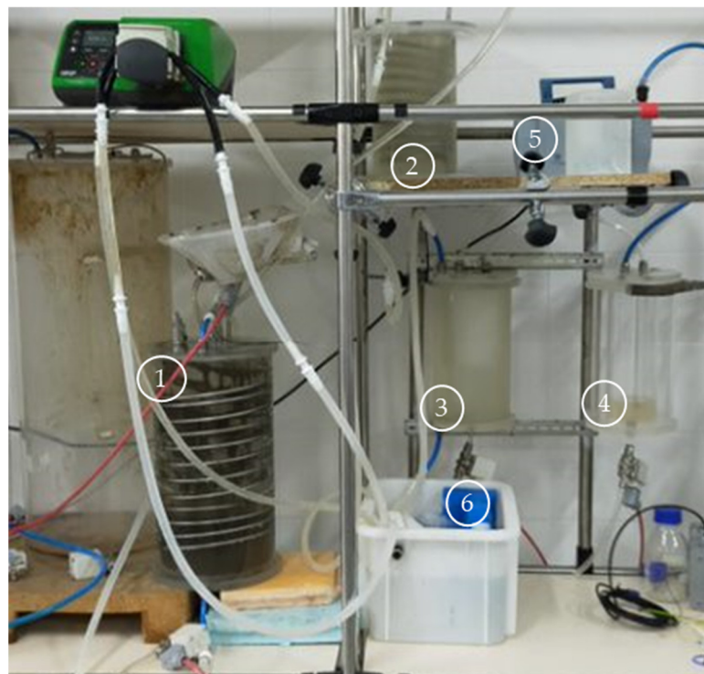
Figure 2. Laboratory-scale low-temperature evaporation set-up: ① evaporator equipped with a heating jacket and heating spiral, ② condenser with a condenser spiral, ③ condensate trapper, ④ acid trap, ⑤ vacuum pump and ⑥ cooling tank.
