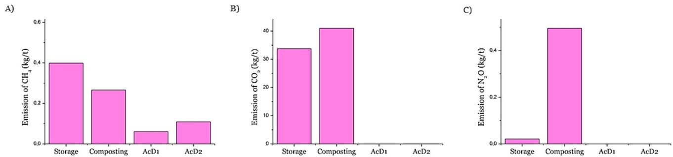
Fig. 9. Emissions of CH<sub>4</sub> (A), CO<sub>2</sub> (B) and N<sub>2</sub>O (C) for four management options: storage of, composting of, anaerobic co-digestion of PM:SS = 60:40 % (VS<sub>added</sub>) with closed digestate storage tank (AcD1), anaerobic co-digestion of PM:SS = 60:40 % (VS<sub>added</sub>) with opened digestate storage tank (AcD2).
